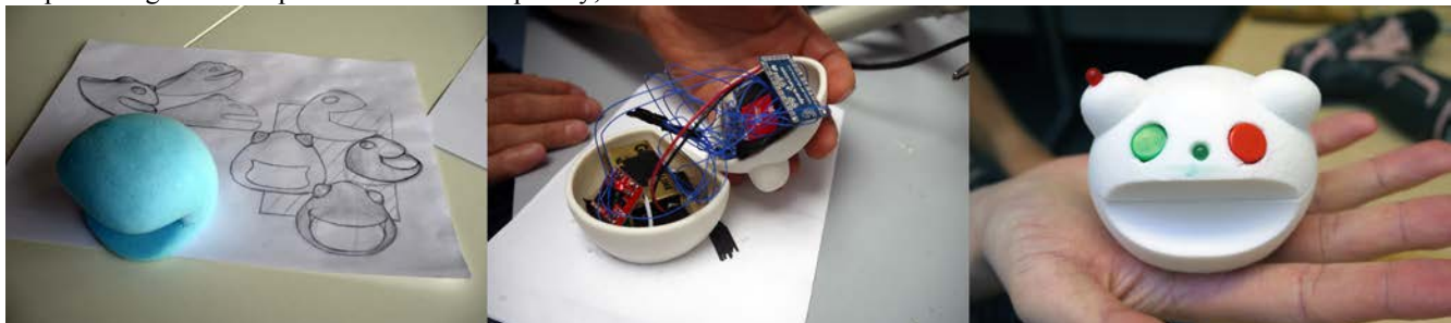
Figure 2 Second Prototype (Left – Blue-form model of 'cat head'; Centre – Embedded electronics of interactive prototype; Right – First interactive prototype)
