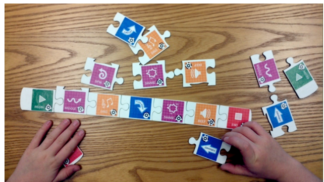
Figure 2. The Tern tangible programming system uses puzzle pieces to allow for the construction of programs.
