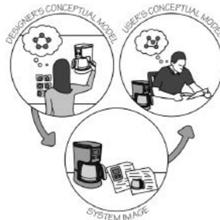
FIGURE 1.11. The Designer's Model, the User's Model, and the System Image.
