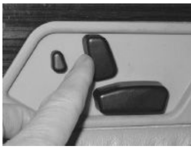
FIGURE 1.7. Good Mapping: Automobile Seat Adjustment Control. This is an excellent example of natural mapping. The control is in the shape of the seat itself: the mapping is straightforward. To move the front edge of the seat higher, lift up on the front part of the button. To make the seat back recline, move the button back. The same principle could be applied to much more common objects. This particular control is from Mercedes-Benz, but this form of mapping is now used by many automobile companies. (Photograph by the author.)
