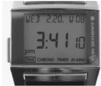
FIGURE 1.8. Junghans Mega 1000 Digital Radio Controlled Watch. There is no good conceptual model for understanding the operation of my watch. It has five buttons with no hints as to what each one does. And yes, the buttons do different things in their different modes. But it is a very nice-looking watch, and always has the exact time because it checks official radio time stations. (The top row of the display is the date: Wednesday, February 20, the eighth week of the year.) (Photograph by the author.)
